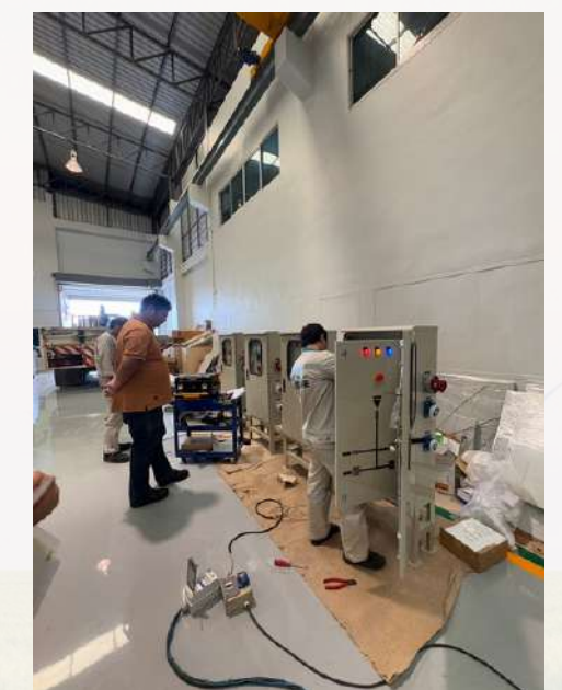
DB Indoor 400 V = 3 panels W600xH1500xD225mm.
