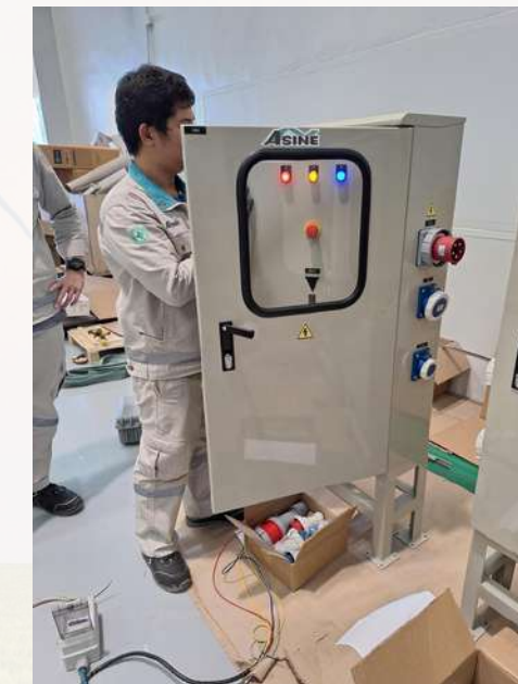
DB Indoor 400 V = 3 panels W600xH1500xD225mm.
